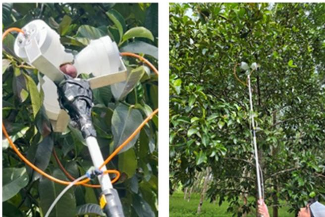
Fig. 17. Operation of mangosteen harvesting equipment: in use during harvesting (left), harvesting at elevated heights (right).
