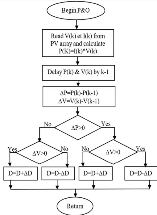
Fig. 3. Flowchart of P&O algorithm.
