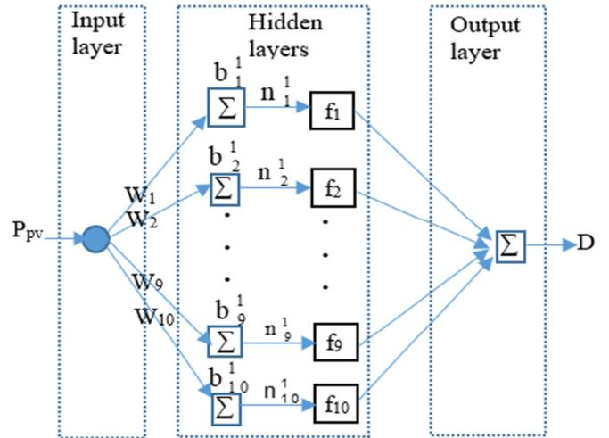
Fig. 4. The proposed neural network architecture.
