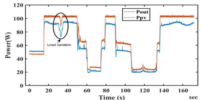
Fig. 13. Experimental power for ANN control under different irradiances.
