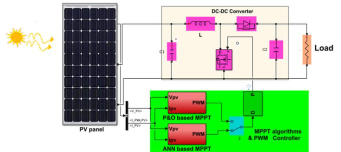
Fig. 1. Block diagram of the studied PV system.
