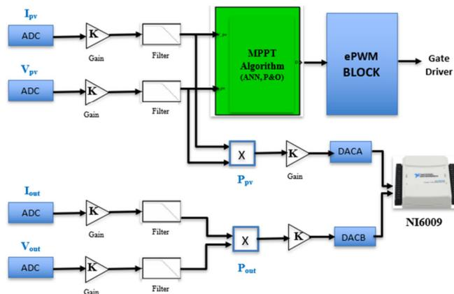
Fig. 11. Program for acquiring data using the DSP F28379D and processing the data with MATLAB-Simulink.
