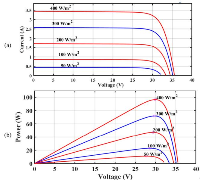
Fig. 2. (a)  $I$ - $V$  and (b)  $P$ - $V$  characteristic curve of PV panel under different levels of solar irradiation and constant temperature of 25°C.
