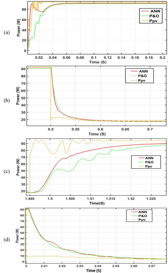
Fig. 9. An approximate comparison of output power using P&O and ANN methods for MPPT :(a) 0 s to 0.2s, (b) 0.4 s to 0.75 s, (c) 1.4 s to 1.53s, (d) 2 s to 2.08 s.
