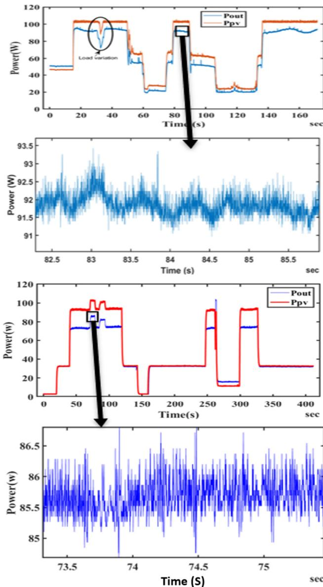
Fig. 15. An approximate comparison of experimental power using P&O and ANN methods for MPPT.
