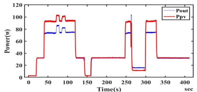
Fig. 14. Experimental power for P&O control under different irradiances.
