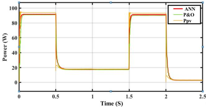
Fig. 8. The generated PV powers by the ANN and the P&O.
