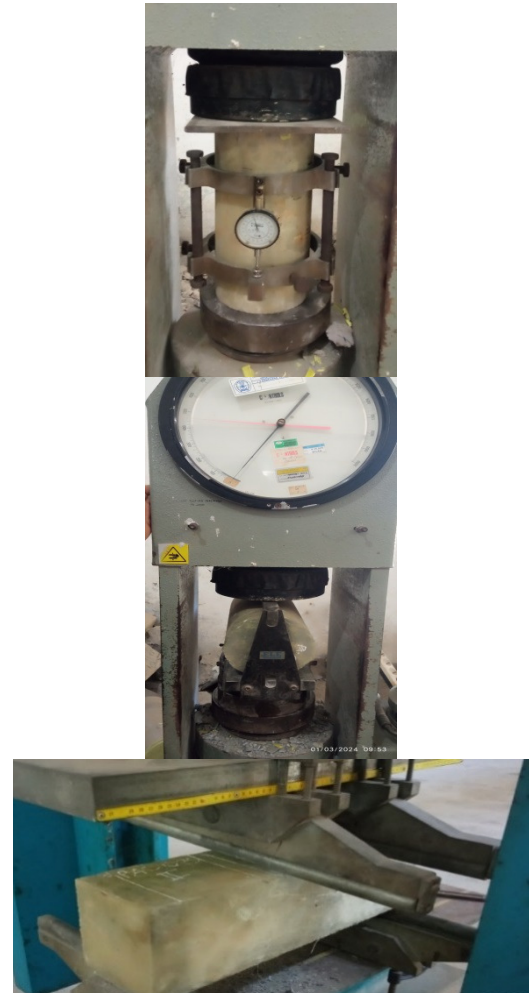
Fig. 6. (a) Compressive strength testing, (b) tensile strength testing, (c) modulus of rupture testing.
