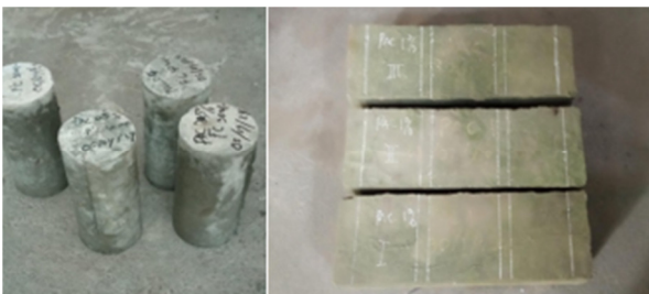
Fig. 4. Cylindrical and prism beam specimens.
