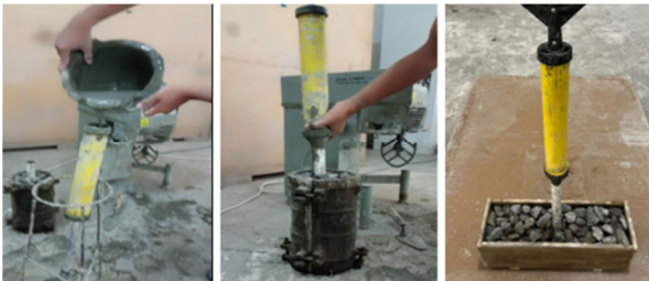
Fig. 3. Grouting pumping process.
