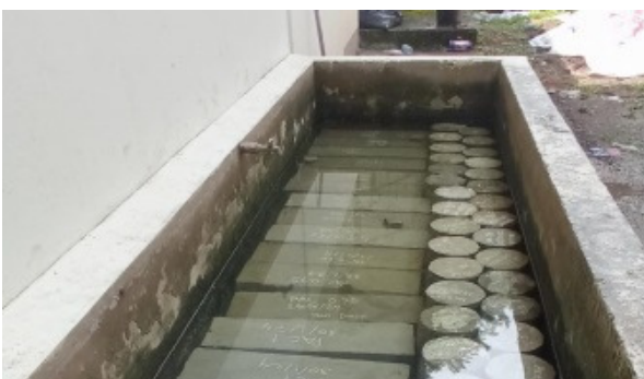
Fig. 5. Curing cylindrical and prism beam specimens.
