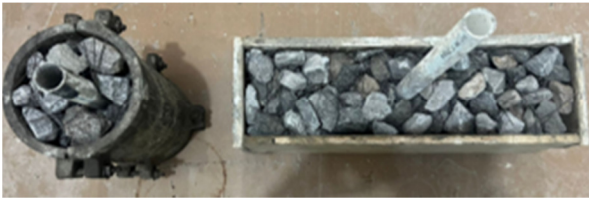
Fig. 2. Placement of coarse aggregate and wire fibers in cylindrical and prism molds.
