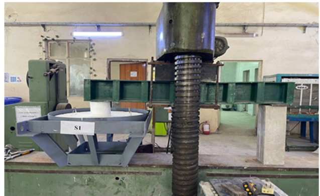
Fig. 3. Slabs under applied load.
