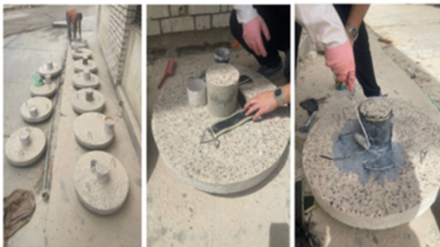
Fig. 2. Applying CFRP sheet to the specimens.
