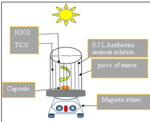
Fig. 2. Diagram of advanced oxidation technology utilizing solar energy.
