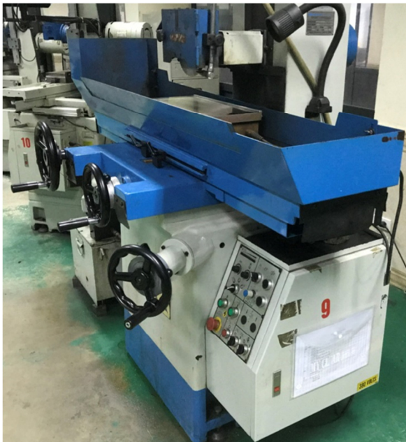
Fig. 2. The ACRA hydraulic surface grinder modeled APSG-820/2A, Taiwan, with a table size of 200 × 500 mm.
