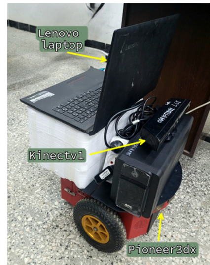
Fig. 4. System implementation of Kinect V1 on the robot Pioneer 3DX.
