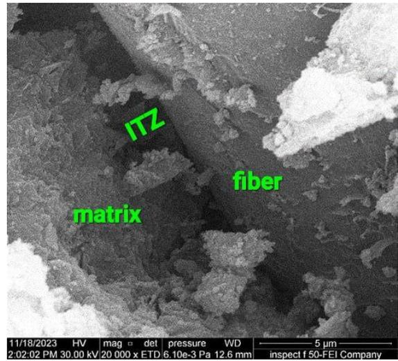
Fig. 4. Bond between matrix and PP fibers (hydrophobic material).
