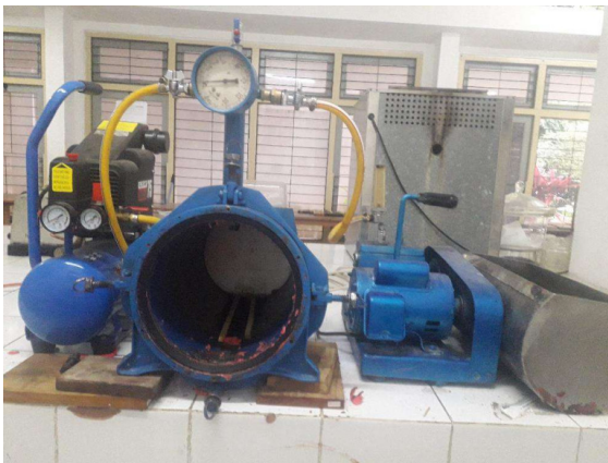
Fig. 1. Wood impregnation equipment.
