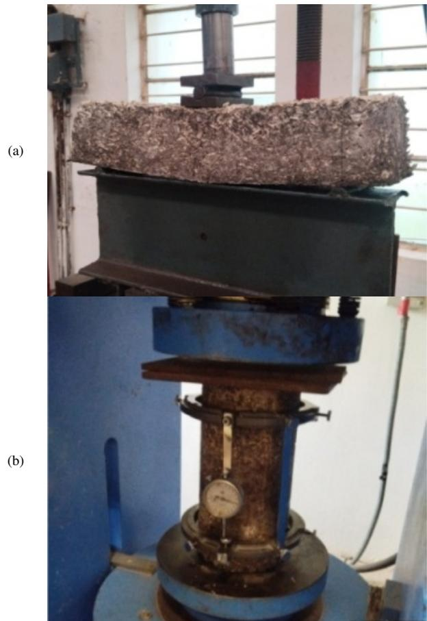
Fig. 8. (a) Flexural strength test setup, (b) Young's modulus test setup.
