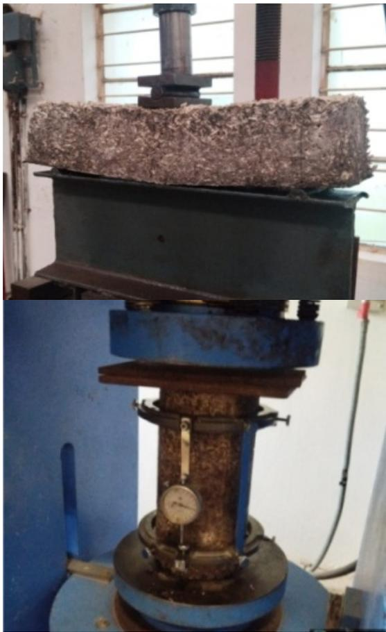
Fig. 2. (a) Flexural strength test setup, (b) Young's modulus test setup.
