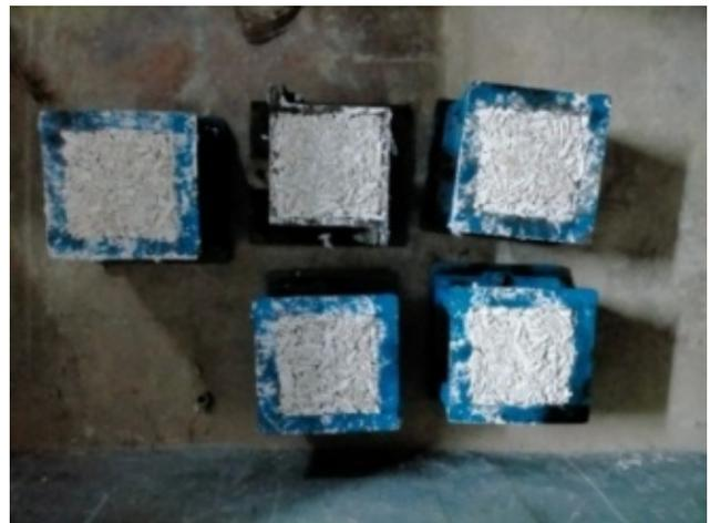
Fig. 1. Hempcrete cubes casted for compressive strength test.
