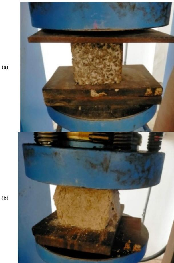
Fig. 5. Typical failure of Hempcrete (a) CAC under compression, (b) LI under compression.
