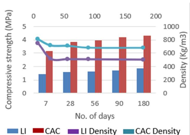
Fig. 7. Relation between compressive strength and density of LI and CAC.
