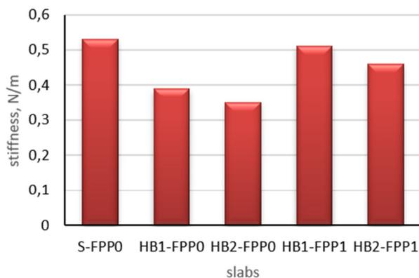
Fig. 7. Average stiffness for all tested slabs.
