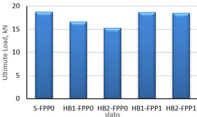
Fig. 5. The effect of voids and PP fibers on ultimate load capacity of all tested slabs.
