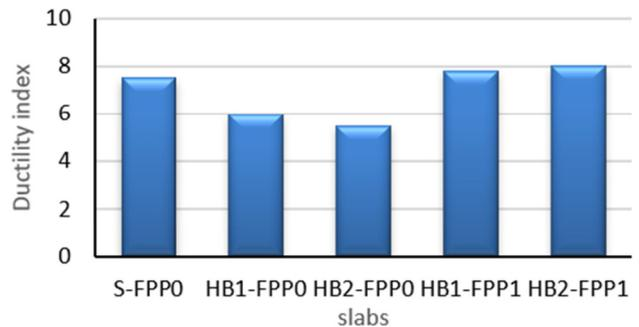
Fig. 6. Ductility indexes for all tested slabs.
