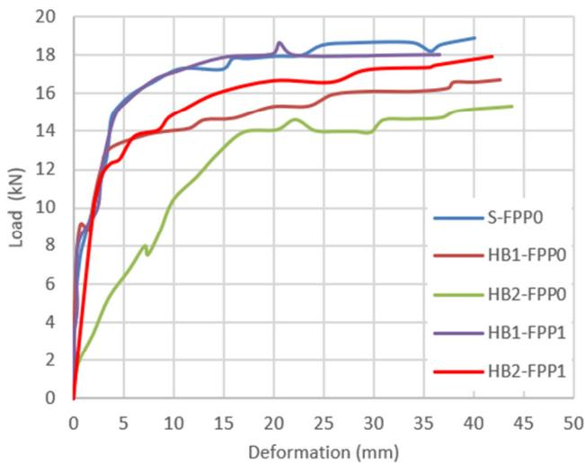
Fig. 4. Load–deflection for all tested slabs.
