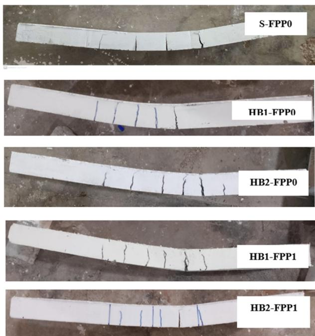
Fig. 8. Crack pattern for all tested slabs.
