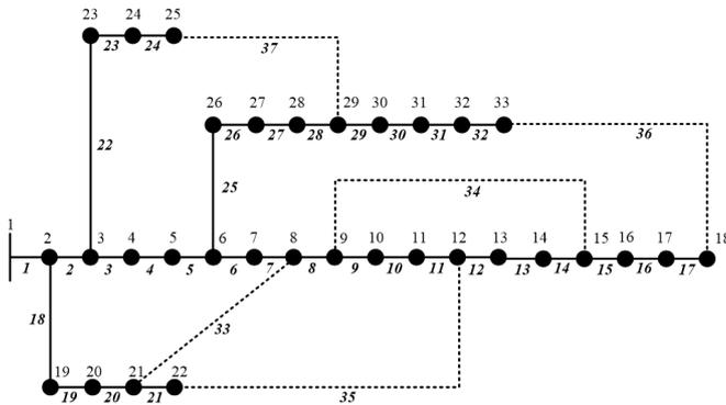
Fig. 1. Single-line diagram of the 33-bus distribution system.
