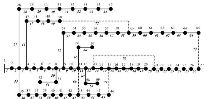
Fig. 3. Single-line diagram of the 69-bus distribution system.
