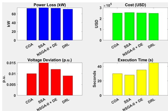
Fig. 2. Comparison of algorithms for the 33-bus system.
