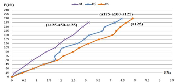
Fig. 7. The L-S relationship of the TZ of the beams.
