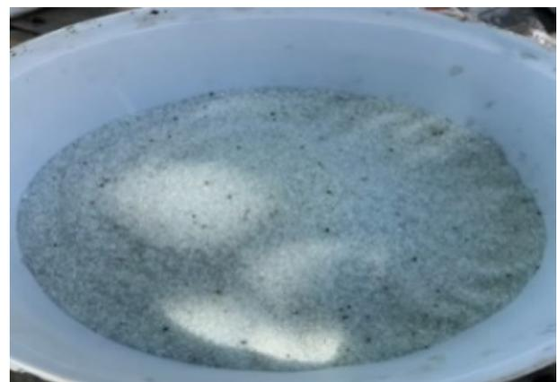
Fig. 1. Produced RG in particle sizes similar to sand particles.
