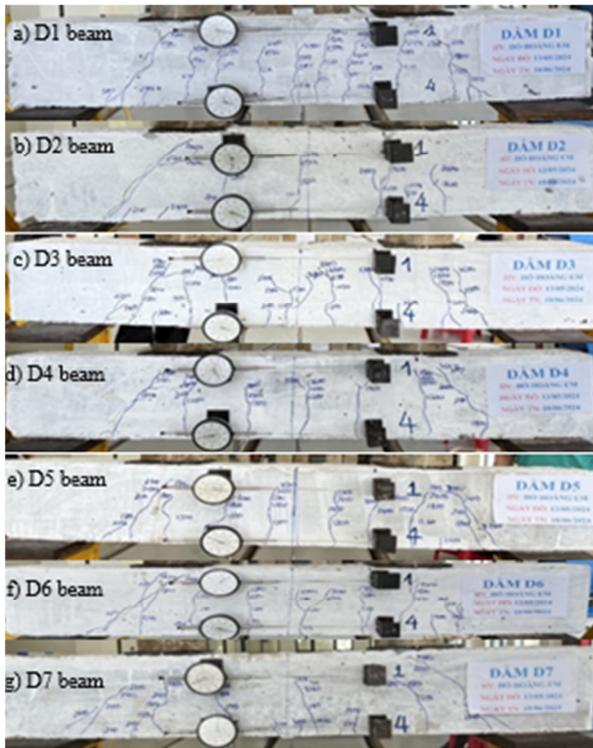
Fig. 2. Crack forming and propagation in the beams
