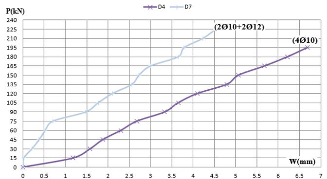
Fig. 11. The L-D relationship of the beams.
