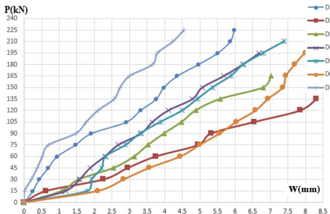
Fig. 14. The L-D relationship of the beams.
