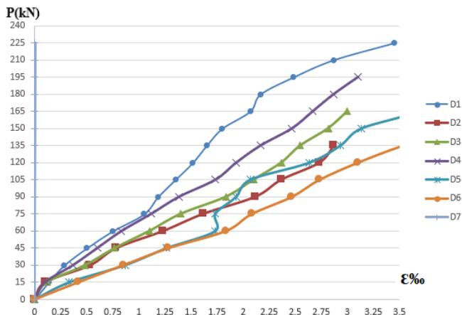
Fig. 13. The L-S relationship of the TZ of the beams.
