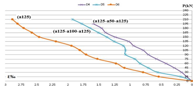
Fig. 6. The L-S relationship of the CZ of the beams.
