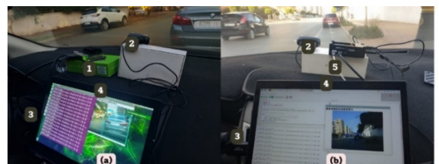
Fig. 2. Experimental setup for embedded deployment: (a) Jetson Nano, (b) Raspberry Pi 5. Components — 1: Jetson Nano, 2: camera, 3: HDMI to USB adapter, 4: Lenovo monitor, 5: Raspberry Pi 5.
