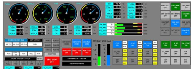
Fig. 5. Engine monitoring interface
