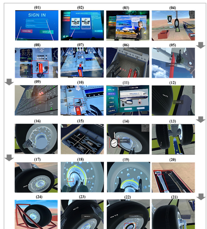
Fig. 10. Procedural flow of the NLG wheel removal simulation.
