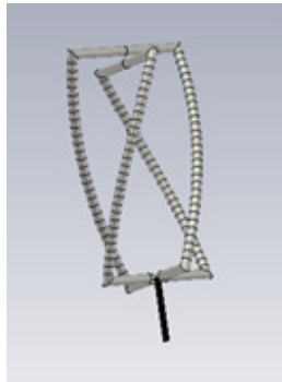
Fig. 1. Simulated antenna in CST.
