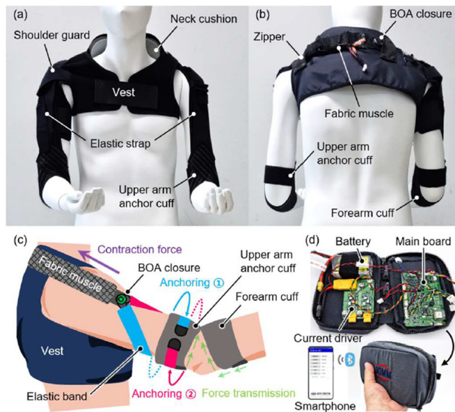
Fig. 7. Soft shoulder exosuit for assisting shoulder elevation in neuromuscular disorders: (a–b) vest-like wearable integrated with elastic straps and fabric-type artificial muscles for comfortable long-term use, (c) conceptual diagram showing contraction force and dual anchoring mechanism for shoulder motion assistance, (d) portable control system including the main board, current driver, and wireless smartphone interface. Reproduced from [26] under CC 4.0 licence [39].
