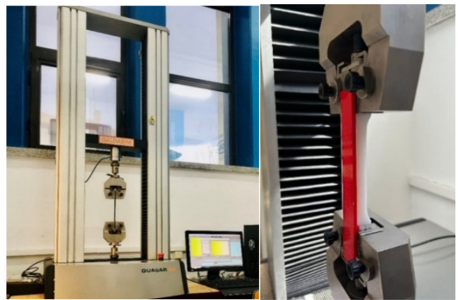
Fig. 2. Test specimen attached to the test machine using the device for positioning and orientation.
