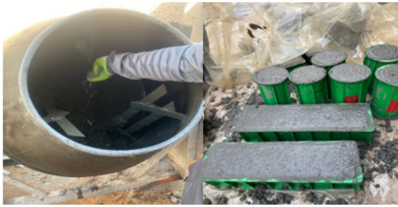
Fig. 7. Casting of concrete mixtures.
