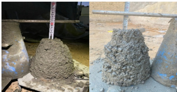
Fig. 8. Workability test of concrete mixtures.
