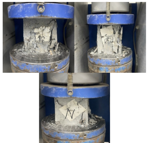
Fig. 9. Compressive performance of concrete mixtures.
