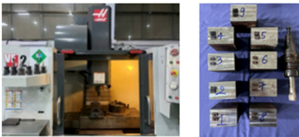
Fig. 1. HAAS CNC milling machine, experimental workpiece, and cutting tools.
