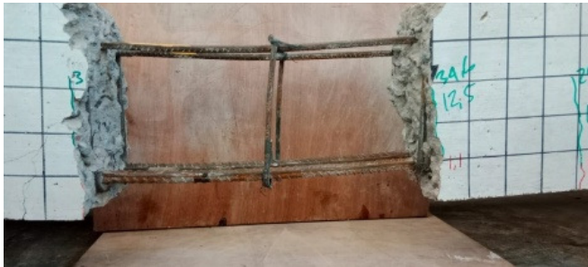
Fig. 13. Residual condition of beam specimen MCB-1.
