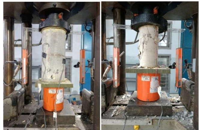
Fig. 5. Testing of confined concrete.
