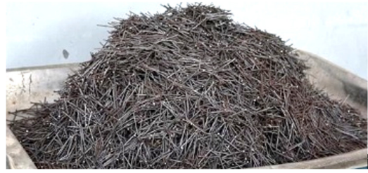
Fig. 1. Image of cut steel fiber.
