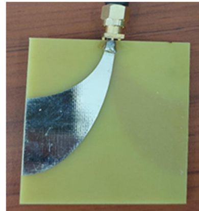
Fig. 2. Top-view of the fabricated microstrip Vivaldi antenna, showing the tapered slot and SMA connector.
