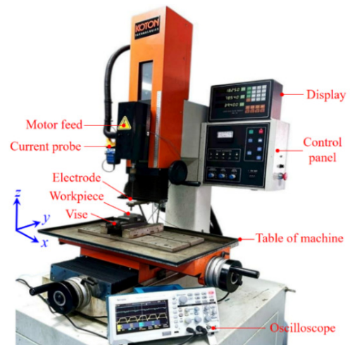
Fig. 1. Experimental setup for small-hole EDM drilling.
