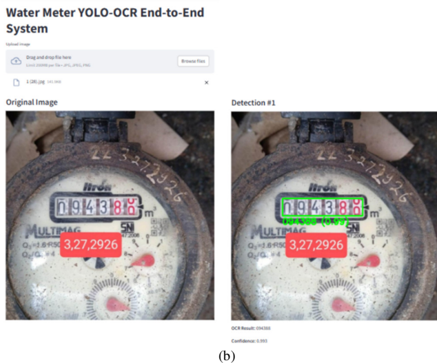
Fig. 9. (a) End-to-end model output visualization, (b) user interface of the developed YOLO-OCR water meter reading system.
