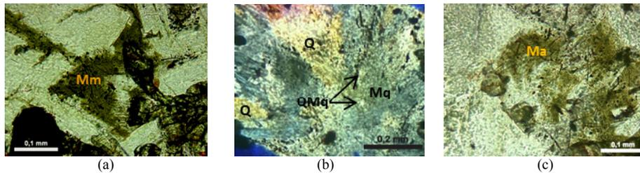
Fig. 3. Micrographs of the mesostasis of the basalt and rhyolite samples, where Mm=microcrystalline mesostasis, Mq=best crystallized mesostasis, Q=matrix quartz, QMq=quartz of the mesostasis, Ma=mesostasis with clay minerals. (a) Mm, natural light, (b) Mq, cross polarized, (c) Ma, natural light. Magnification 20x.
