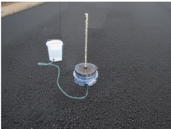
Fig. 4. Field permeability test setup.
