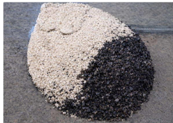
Fig. 3. TGP composite for filling the potholes.
