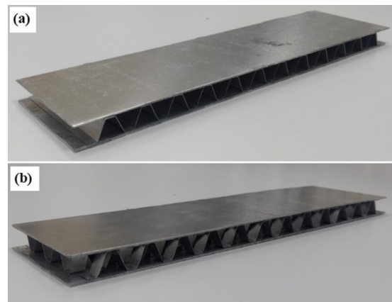
Fig. 4. Experimental samples of metallic sandwich panels: (a) CMC and (b) CSC
