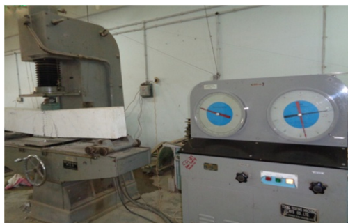
Fig. 4. Short term testing of RC beams
