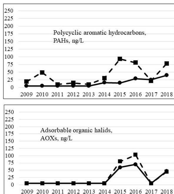
Fig. 5. Evolution per year of: PAHs (up); AOXs ( $\mu\text{g/L}$ ) (down). Raw wastewater (squares-striped line); treated wastewater (dots-continuous line).
