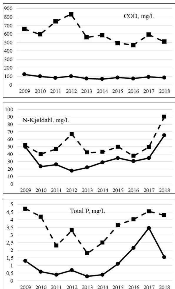
Fig. 3. Evolution per year of: COD (up); Kjeldahl N (middle); Total P (down). Raw wastewater (squares-striped line); treated wastewater (dots-continuous line).
