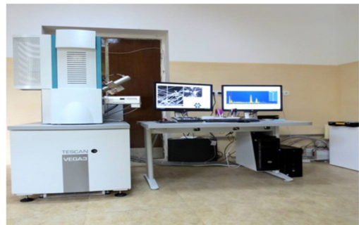
Fig. 2. SEM VEGA3 equipped with EDS of Oxford Instruments
