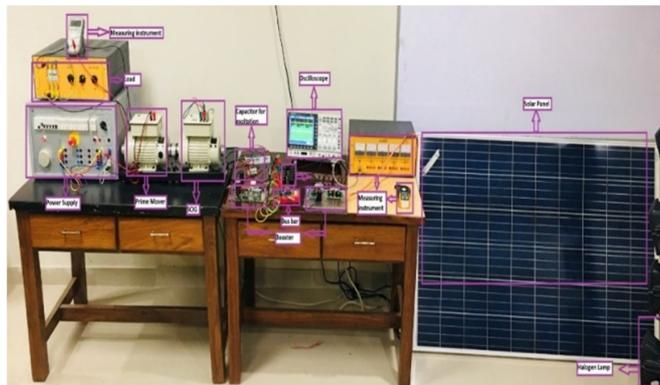
Fig. 8. Experimental model setup for the hybrid power system.
