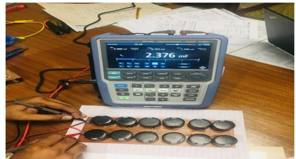
Fig. 7. Super capacitor bank.
