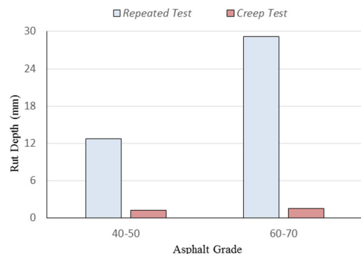
Fig. 9. Asphalt grade vs predicted rut depth on AC layer at 40°C (VESYS 5W analysis).
