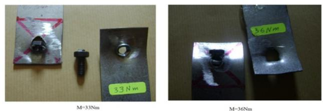
Fig. 14. Mode of rupture for  $M=33Nm$  and  $M=36Nm$ .
