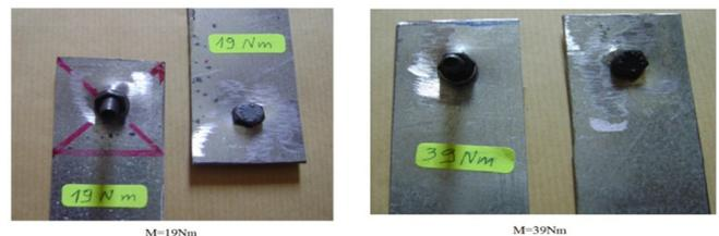
Fig. 13. Mode of rupture for  $M=19Nm$  and  $M=39Nm$ .
