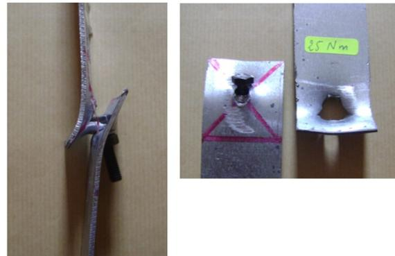
Fig. 12. Mixed tensile-shear failure mode.
