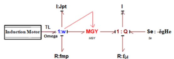
Fig. 20. Bond graph model of the centrifugal pump.
