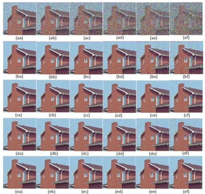
Fig. 4. (aa–af) Hut images corrupted by 20-70%, restored images using: (ba–bf) MF, (ca–cf) NAFSM, (da–df) DBUTVF, (ea–ef) proposed method.
