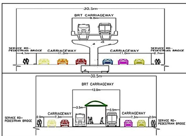
Fig. 3. Gurumandir-Golimar cross-section with existing elevated (top) and proposed median (bottom) alignment.
