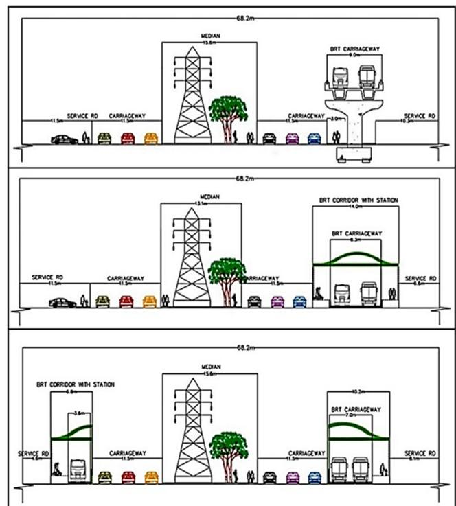
Fig. 4. Nagan-Surjani cross-section with existing elevated alignment (top), proposed two-way side alignment (middle), and curb-side (bottom).
