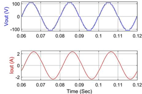
Fig. 7. Output Voltage and current at  $R=100\Omega$  and  $L=63.7mH$  at  $m=0.6$ .
