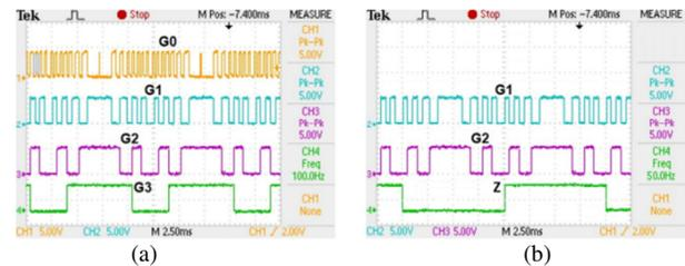
Fig. 9. Generated gate pulses using ADC: (a) Gate pulses of half-bridges, (b) gate pulse of the full h-bridge.
