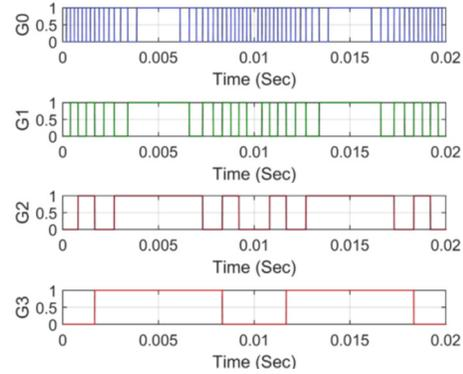
Fig. 5. Output gate pulses from Matlab function block.
