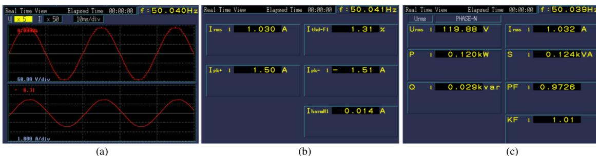
Fig. 10. Prototype hardware results for R= 110Ω and L=63.7mH at modulation index m=1: (a) Output Voltage and current, (b) RMS value and THD of the output current, (c) pf, active, and reactive power.
