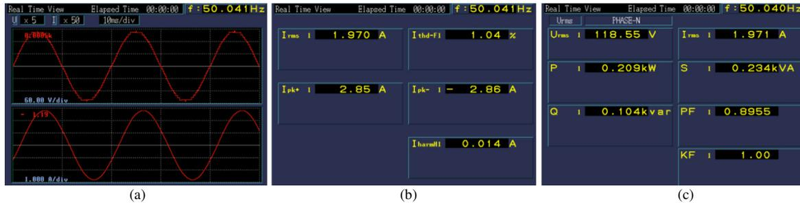
Fig. 12. Prototype hardware results for  $R=60\Omega$  and  $L=63.7\text{mH}$  at modulation index  $m=1$ : (a) Output Voltage and current, (b) RMS value and THD of the output current, (c) pf, active, and reactive power.
