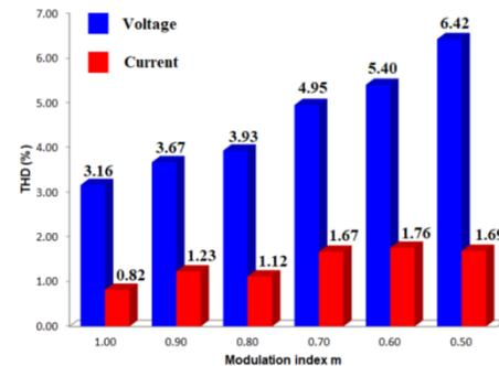
Fig. 8. THD (%) of the output voltage and load current with different values of  $m$ .
