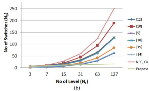
Fig. 3. Comparison graph of the proposed and other topologies: (a) No. of DC sources vs no. of levels, (b) no. of switching devices vs no. of levels.
