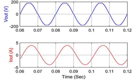
Fig. 6. Output Voltage and current at  $R=42\Omega$  and  $L=63.7mH$  at  $m=1.0$ .
