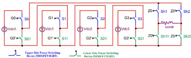
Fig. 1. Power topology of the 31-level MLI.
