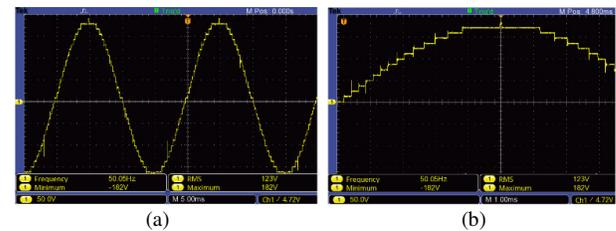
Hardware prototype results of the ADC-controlled 31-level inverter: (a) Output Voltage, (b) zoomed view.
