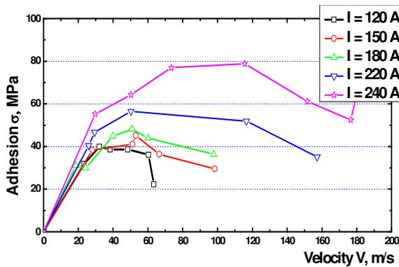
Fig. 2. Relation between adhesion, plasma power, and particle velocity.
