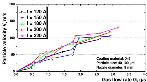
Fig. 3. Relation between particle velocity, plasma power, and air flow rate.
