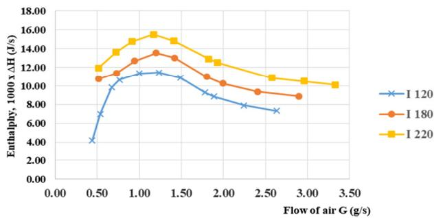
Fig. 1. Relation between enthalpy, plasma power, and air flow rate.
