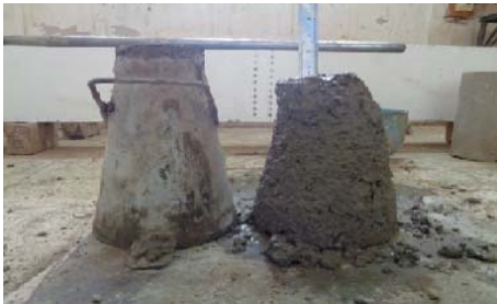
Fig. 6. Slump cone test.
