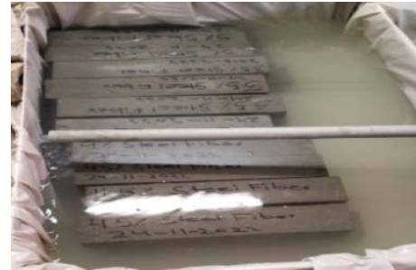
Fig. 7. Specimens and curing.
