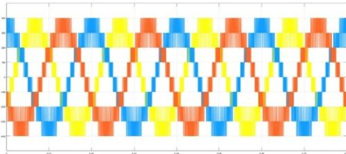
Fig. 17. Line voltages of cascaded MLI with MCPWM.
