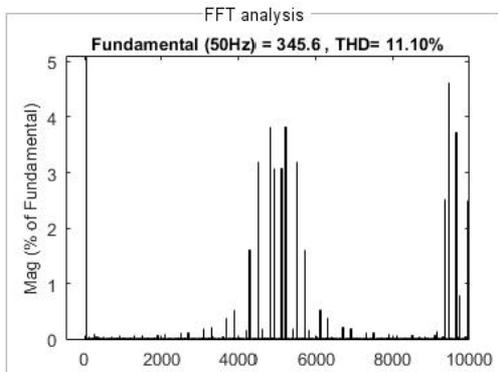
Fig. 10. FFT analysis of diode-clamped MLI with MCPWM.
