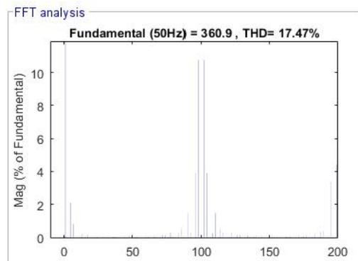
Fig. 14. FFT analysis of cascaded MLI for SPWM.
