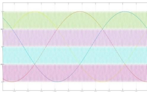
Fig. 1. Sinusoidal reference comparison with normal triangular waves.
