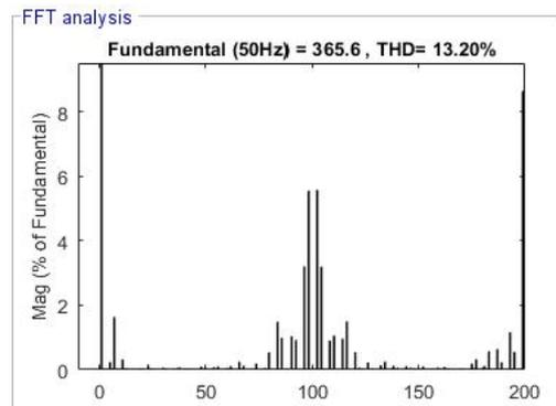
Fig. 8. FFT analysis diode-clamped MLI with MRWM.
