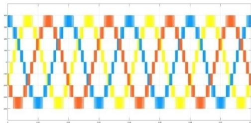
Fig. 5. Line voltages of diode-clamped MLI with SPWM.
