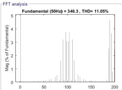
Fig. 18. FFT analysis of cascaded MLI with MCPWM.
