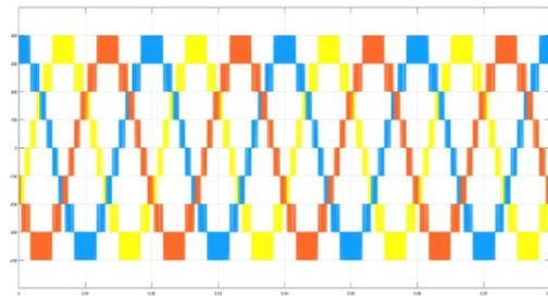
Fig. 7. Line voltages of diode-clamped MLI with MRWM.
