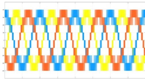
Fig. 9. Line voltages of diode-clamped MLI with MCPWM.
