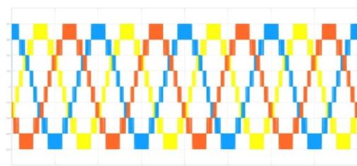
Fig. 15. Line voltages of cascaded MLI with MRPWM.
