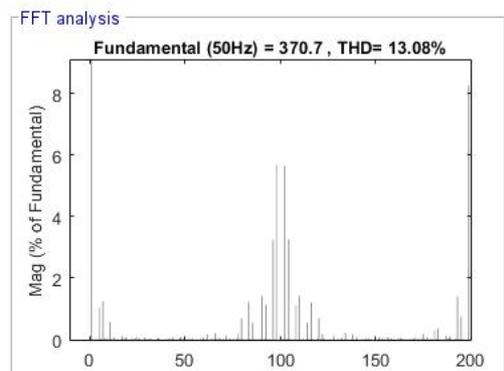
Fig. 16. FFT analysis of cascaded MLI with MRPWM.
