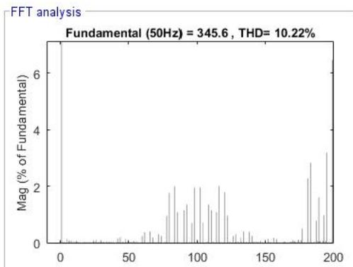
Fig. 12. FFT analysis of diode-clamped MLI with MRMCPWM.
