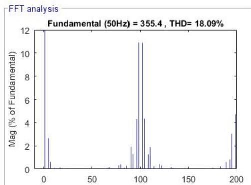
Fig. 6. FFT analysis of diode-clamped MLI with SPWM.
