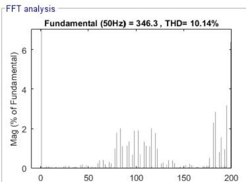
Fig. 20. FFT analysis of cascaded MLI with MRMCPWM.
