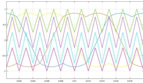
Fig. 4. Modified reference comparison with modified carrier waves.
