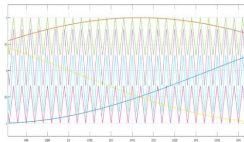
Fig. 3. Sinusoidal reference comparison with modified carrier waves.
