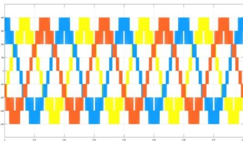
Fig. 19. Line voltages of cascaded MLI with MRMCPWM.
