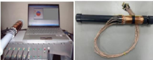
Fig. 8. Typical 12-electrode ECT sensor setup and ECT system.
