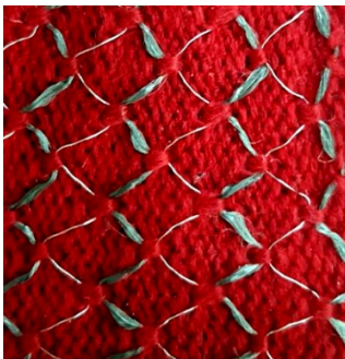
Fig. 8. Stainless steel yarn and wire of 0.15 mm diameter.
