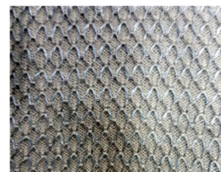
Fig. 5. A sample using stainless steel and tungsten yarns.
