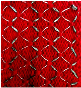
Fig. 7. Silver enriched yarn with stainless steel wire of 0.15 mm diameter.
