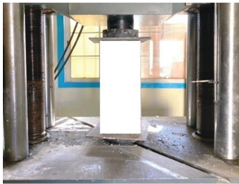
Fig. 3. Testing of concrete columns by UTM load compression.
