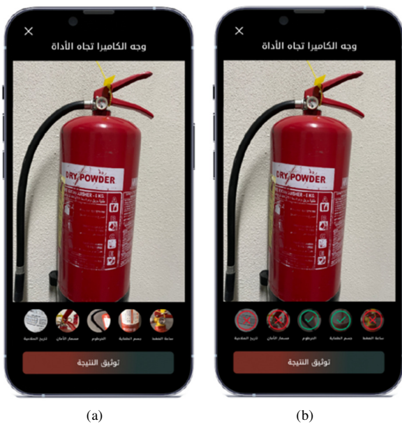
Fig. 7. Weqaa interfaces: (a) Camera pointed at equipment, (b) detection results.
