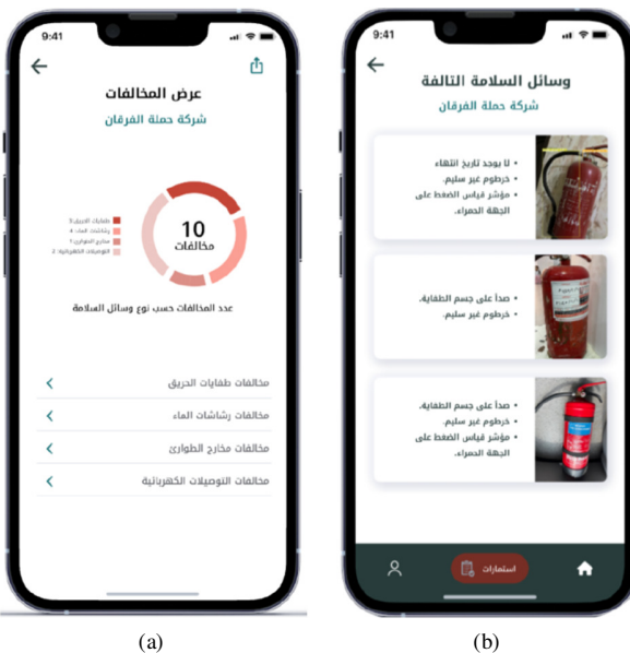
Fig. 12. Weqaa Interfaces: (a) Violations statistics, (b) detected violations.
