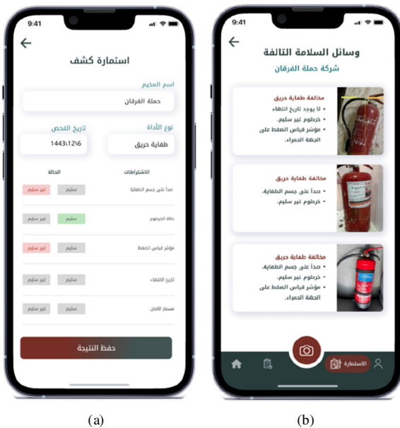
Fig. 8. Weqaa interfaces: (a) Confirm inspection result, (b) all defective equipment at one location.
