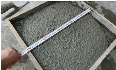
Fig. 3. T 500mm test.
