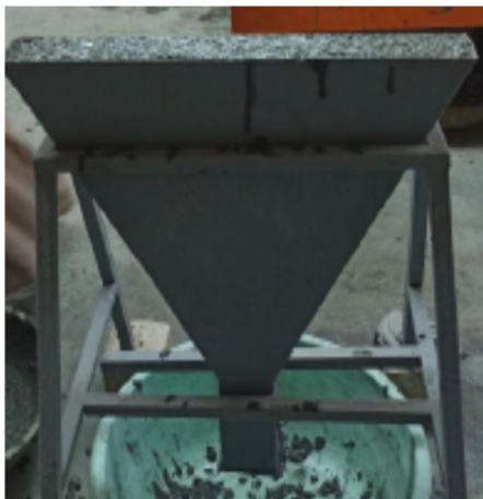
Fig. 4. V-Funnel time test.
