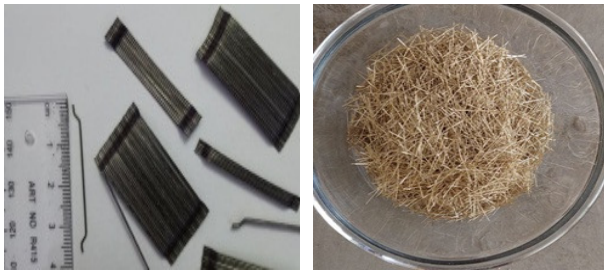
Fig. 1. The two types of steel fibers used.
