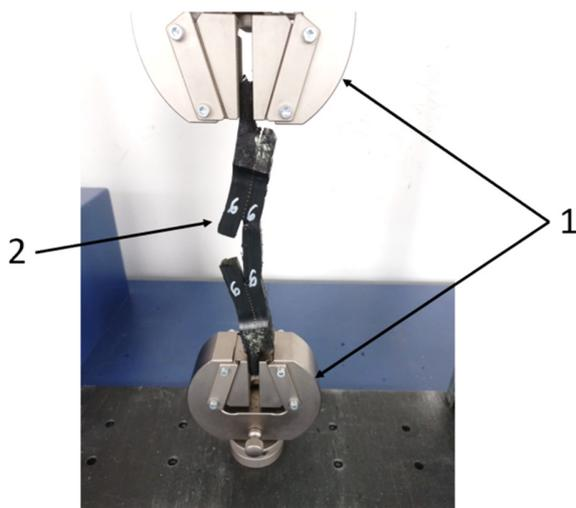
Fig. 4. Tensile strength testing on the Mecmesin Multitest 10-i universal testing machine: 1- pans; 2- welded sample.
