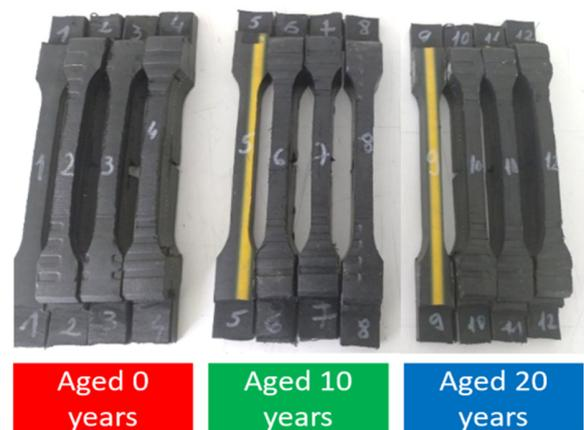
Fig. 3. Tensile samples made of PE100 SDR11.
