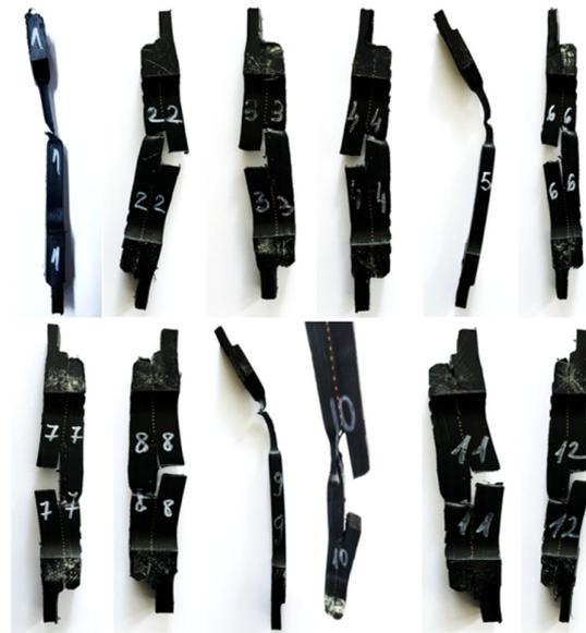
Fig. 5. PE100 SDR 11 samples after tensile strength testing.
