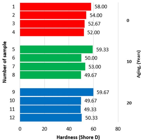
Fig. 12. Average Shore D hardness values for PE100 SDR11 samples.
