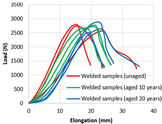
Fig. 7. Tensile strength test charts of welded samples.
