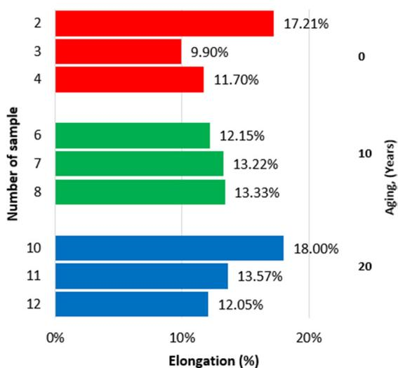
Fig. 9. Percentage elongation values obtained at the breakage of tensile strength tested welded samples.
