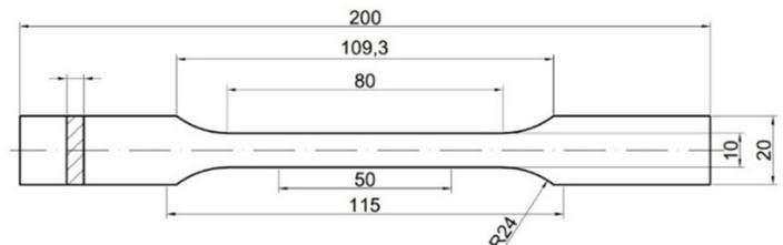
Fig. 2. Tensile sample model, type 1A.
