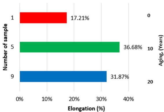
Fig. 8. Percentage elongation values obtained just before the breakage of the unwelded samples in the tensile strength tests.
