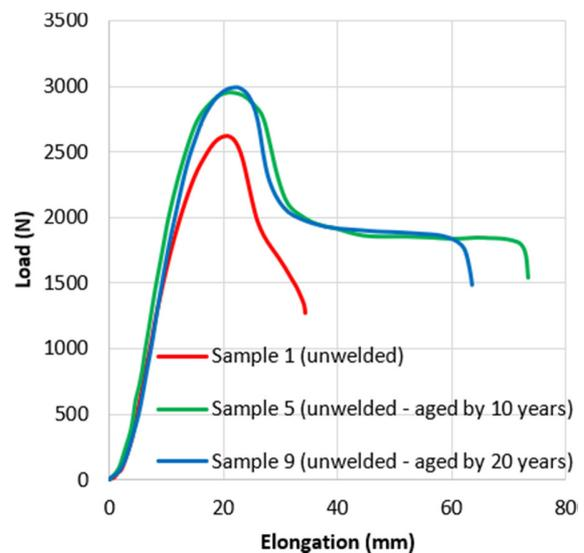
Fig. 6. Tensile strength test charts of unwelded samples.
