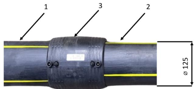
Fig. 1. The PE100 SDR11 pipe welded by electrofusion. The arrows 1 and 2 point to the pipes and arrow 3 points to the welded assembly.
