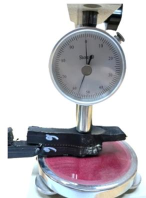
Fig. 11. The Shore D analogue hardness tester.
