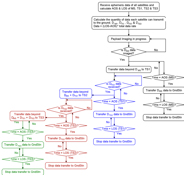
Fig. 4. Scenario-1 flowchart for satellite identification and data transfer.
