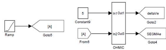
Fig. 18. The electrolyzer Ohmic potential model
