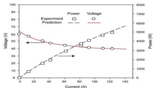
Fig. 12. Values for current, voltage and output power in the polarization curve of experimental and predicted results
