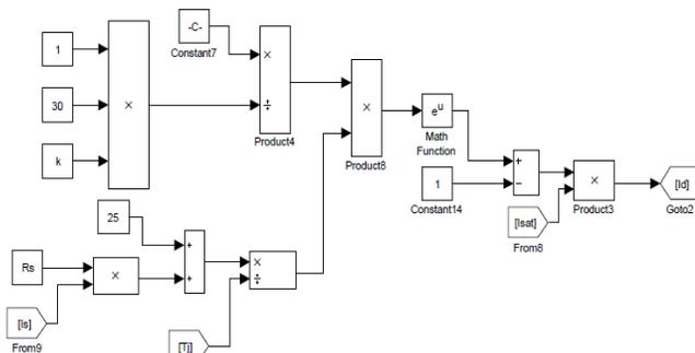
Fig. 2. The PV diodes losses model
