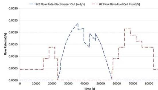
Fig. 20. Velocity of hydrogen flow at the times of production and consumption via electrolyzer and fuel cell
