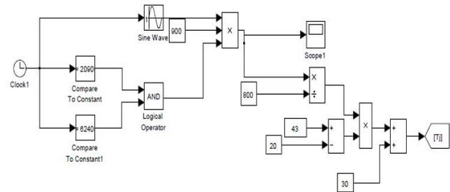
Fig. 6. The model of ambient air and PV cells' heat
