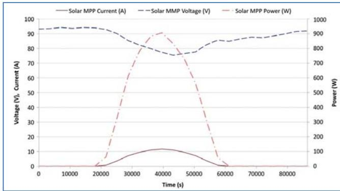
Fig. 8. Graph of output current, voltage and power generated by the solar cell during a day
