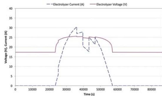
Fig. 19. Electrical dynamics of the electrolyzer system
