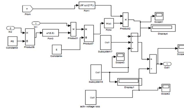
Fig. 11. The hydrogen storage tank system model
