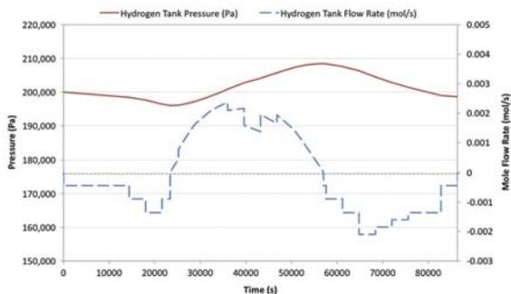
Fig. 21. Volume of the hydrogen flow and pressure alterations in the liquid hydrogen tank at the times of storage and consumption
