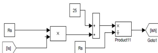
Fig. 4. The PV shunt current model
