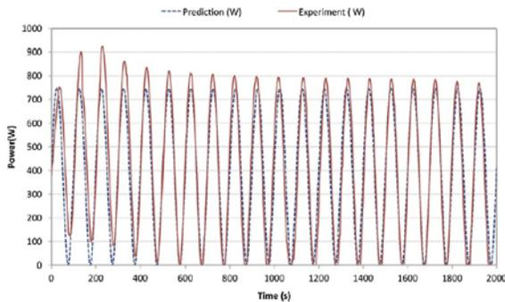
Fig. 14. Comparison of the predicted output power and the response of the output power measured from the fuel cell system at the same conditions
