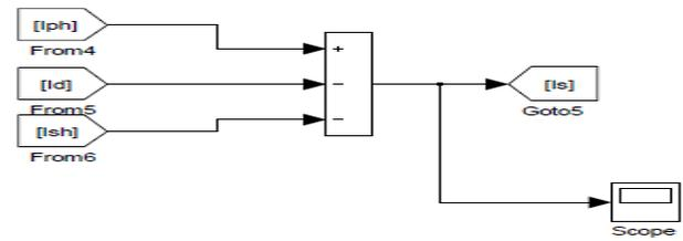
Fig. 5. The PV overall current output model
