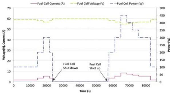
Fig. 15. Values of the current output, voltage and power at during turning on and off of the fuel cell system
