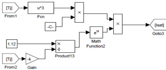
Fig. 1. The PV saturated currents model
