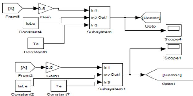
Fig. 16. The model of the actual voltage in the electrolyzer system
